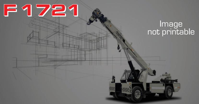
Capacity 17 T I Boom Height with Fly Jib 21 M I Snatch Block Heavy Duty (6 Falls) Creep Speed 1.3 kmph I Structure Heavy Duty I Speed 49 kmph
