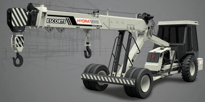
Capacity: 12 T I Boom Height: 36 Feet I Service Interval Engine: 500 hrs. I Straight Axle: Heavy Duty I Transmission: Robust (8+2)
