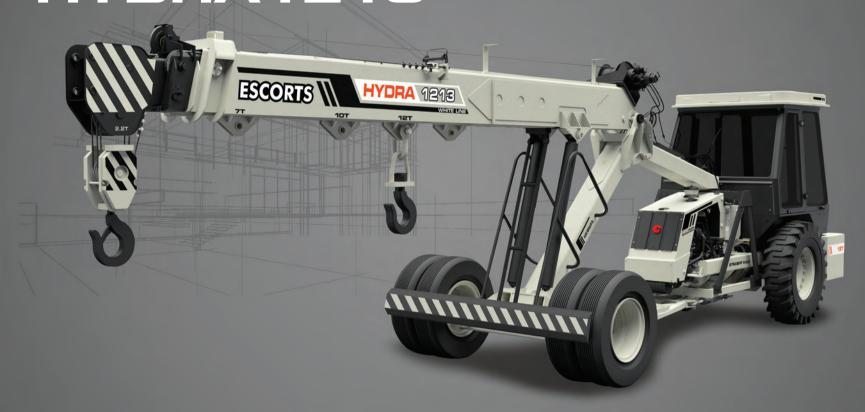
Capacity: 12 T I Boom Height: 42 Feet I Service Interval Engine: 500 hrs. I Straight Axle: Heavy Duty I Transmission: Robust (8+2)
