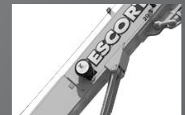
SLI – Safe Load Indicator
