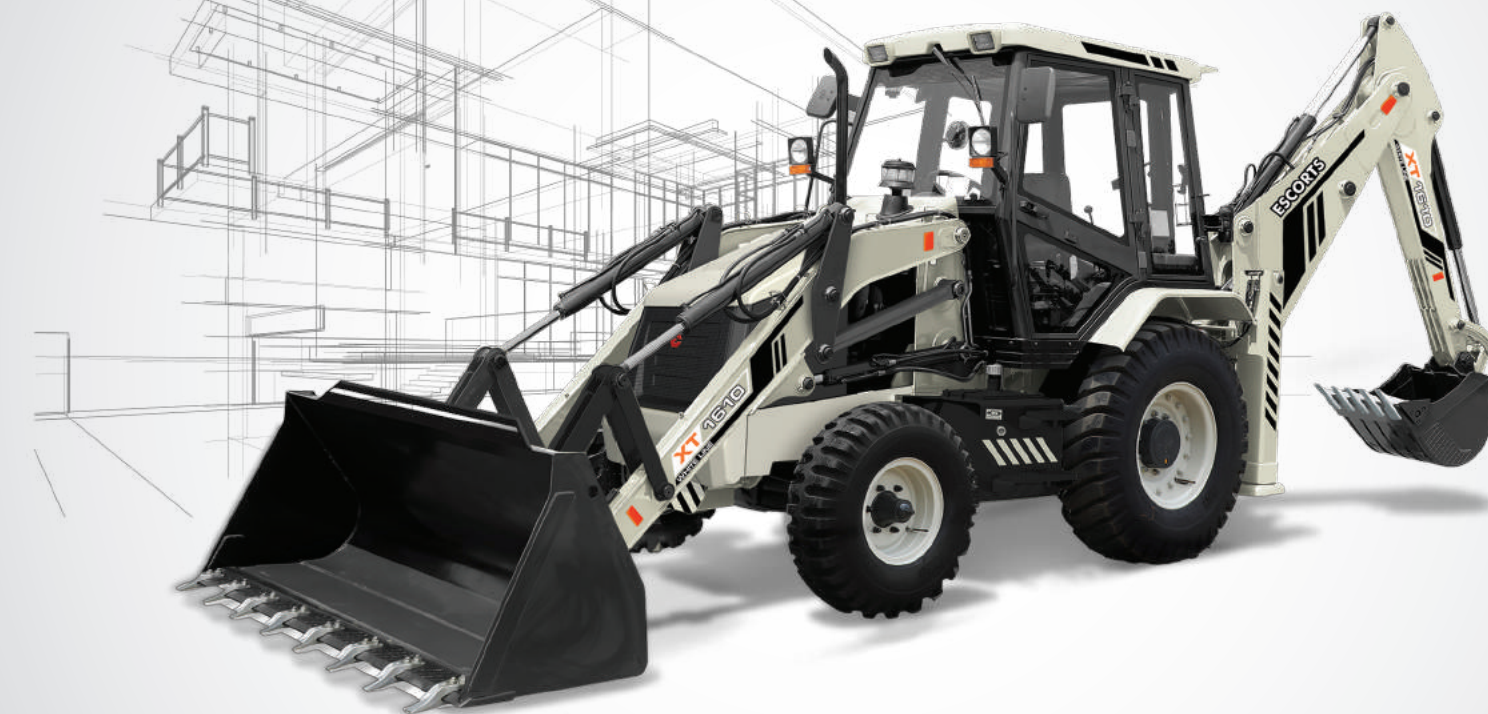
Escorts Engine: 75 HP | Max. Dig Depth: 4.8 m | Load Over Height: 3.51 m
